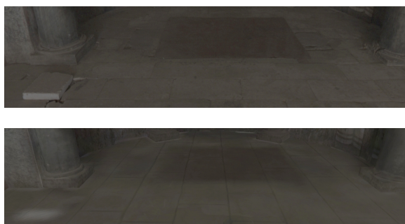
Figure 9: Examples of where IBS is useful for 3D model accuracy assessment. Two problems became apparent when comparing the virtual model (bottom) to a photograph (top). Firstly, the floor texture coordinates are incorrect, leaving the floor bricks to face the wrong direction. Secondly, the brick tile on the left hand side of the photograph is not modelled, showing up as incorrect bright splats.
